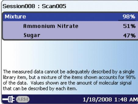
Advanced mixture analysis algorithms enable accurate identification of solid/liquid combinations and aqueous, organic solvent and other solutions.
