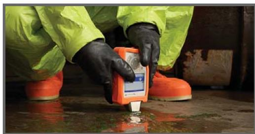
**TruDefender™ FT** is a rugged, handheld FTIR system for rapid, in-the-field identification of unknown chemicals. Unlike other instruments available today, TruDefender FT brings the power of FTIR directly into the hotzone, enabling the responder to analyze - and act - faster than ever before.
