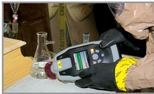
**FirstDefender®** is deployed worldwide for rapid, accurate identification of unknown chemicals. Designed to meet the needs of first responders, FirstDefender is a lightweight, rugged instrument that increases responder safety and delivers precise results in seconds.
