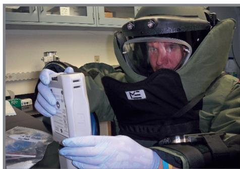
**TruDefender™ FT** is a rugged, handheld FTIR system for rapid, in-the-field identification of unknown chemicals including explosives, narcotics and white powders. Unlike other instruments available today, TruDefender FT brings the power of FTIR directly into the field, enabling law enforcement personnel to analyze—and act—faster than ever before.
