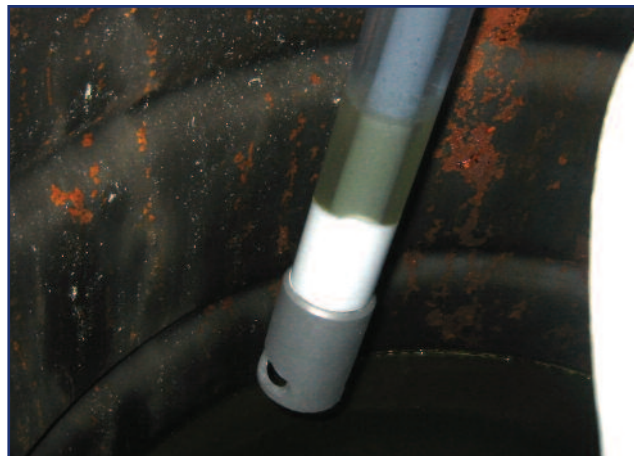
Figure 2: COLIWASAs are used to sample stratified wastes in a container.
