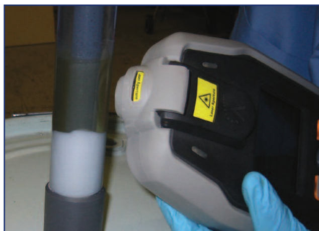
Figure 3: Each layer of the stratified waste contained in a COLIWASA is rapidly identified by Ahura's First Defender unit.
