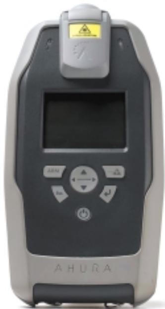
sample. Therefore, the sample does not need to be moved or collected to perform rapid and accurate on-the-spot analysis. The Defender can be used to positively identify the material in question.
